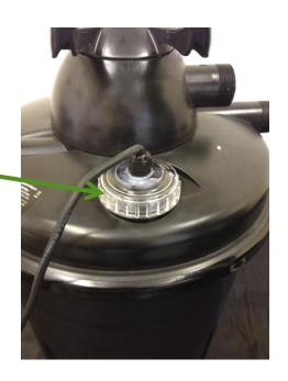
Be careful when removing this piece as the bulb occasionally falls from this fitment; this can be easily retrieved from the bulbs housing; the quartz sleeve.
